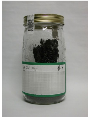
Figure 3: Glass Mason jar with fire debris.
